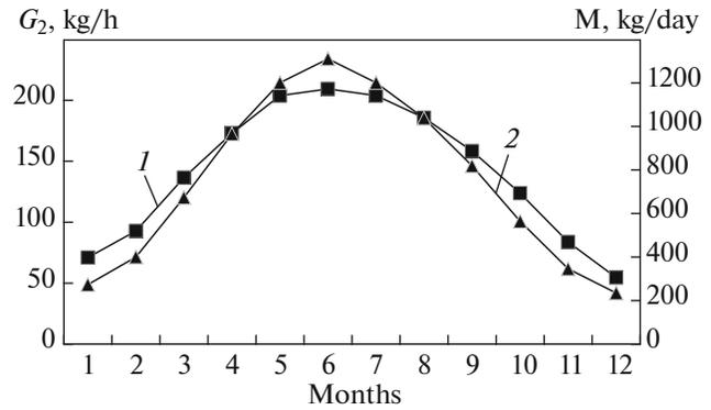
Fig. 6. Schedule of the (1) hourly consumption and (2) storage of the daily amount of heated water.
