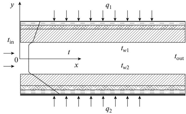
Fig. 2. Scheme of calculating the heat-transfer fluid temperatures in the channels of the solar cell.
