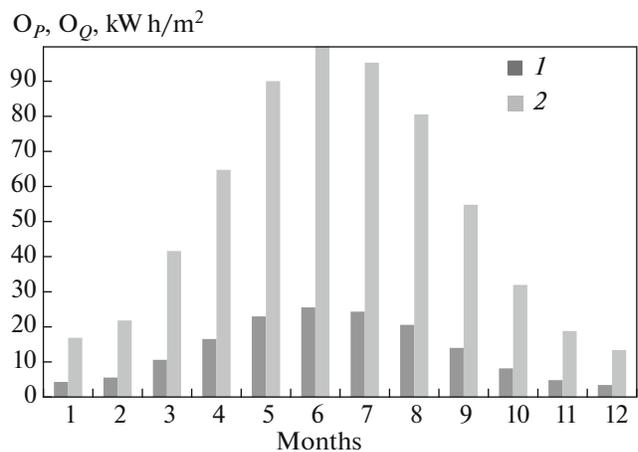
**Fig. 5.** Average monthly specific (1) electricity and (2) heat output of the cogeneration plant.
