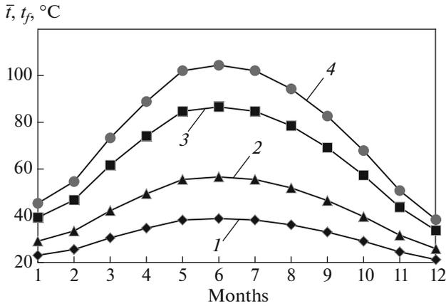
Fig. 4. Mean integral heat-transfer fluid temperatures in (1) channel 1 and (3) channel 2 and of the solar cells in (2) channel 1 and (4) channel 2 at  $G = 150$  kg/h.
